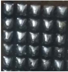
Fig 3. 5x5 capacitive Sensor Array
