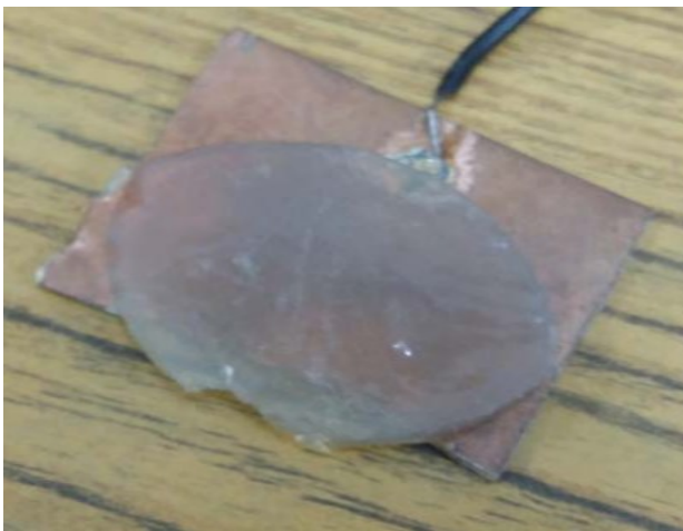
Fig 4. The prepared Agar-Agar phantom.
